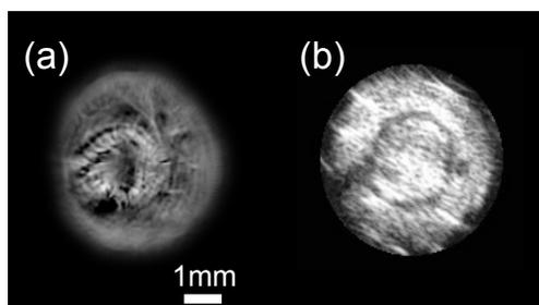
Fig. 1. Cross-sectional images of *Lumbricus Terrestris*. (a) Optoacoustic image made at 750 nm; (b) The corresponding ultrasound image acquired using high-resolution ultrasound imaging system operating at 25MHz.
